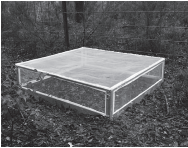
Fig. 1. Predator exclusion cage designed for the field experiment directed to estimate the acorn manipulation rates by Thorectes baraudi and Jekelius nitidus . These cages are wooden squares (1 × 1 × 0.3 m) covered with a protective stainless steel mesh (0.25-cm grid size) that hinder acorn predation by rodents, birds, and other insects. The cages were placed within wider fenced areas to exclude red deer, roe deer, and wild boar.
